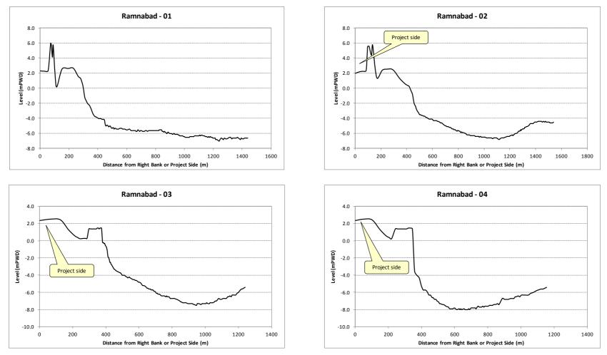
Figure 6-21: Surveyed Cross-Sections of the Rabnabad Channel
