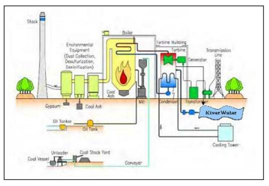
Figure 3-4: Typical diagram of coal fired thermal power plant
