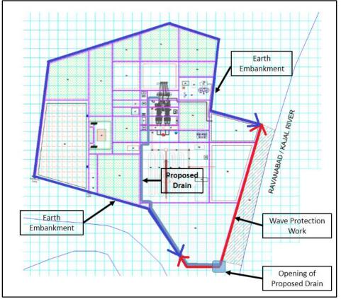
Figure 3-8: Protection Work of River/Canal Banks for Project Area
